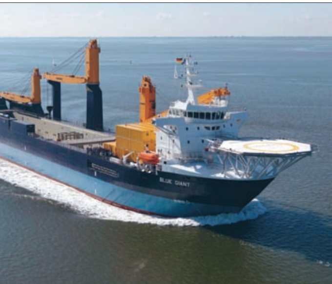
The Blue Giant, equipped with helicopter landing deck, cabins for 200 workers and a bell for operations in a water depth of 200 m.
