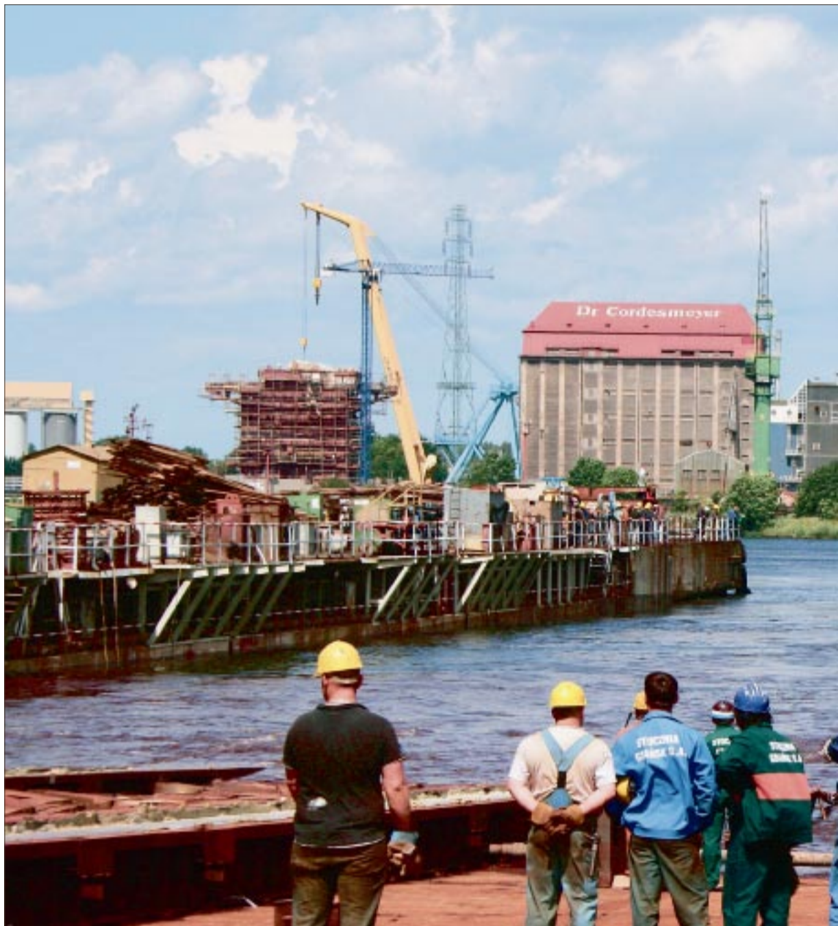
READY: The 11,000-dwt multifunction heavylift "Combi Dock IV" slides down the slipway
