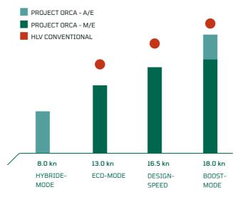
"Compared to conventional heavy lift vessels, fuel consumption is 45% lower in eco mode (13kn) and approx. 33% lower in cruise speed (16kn)."
